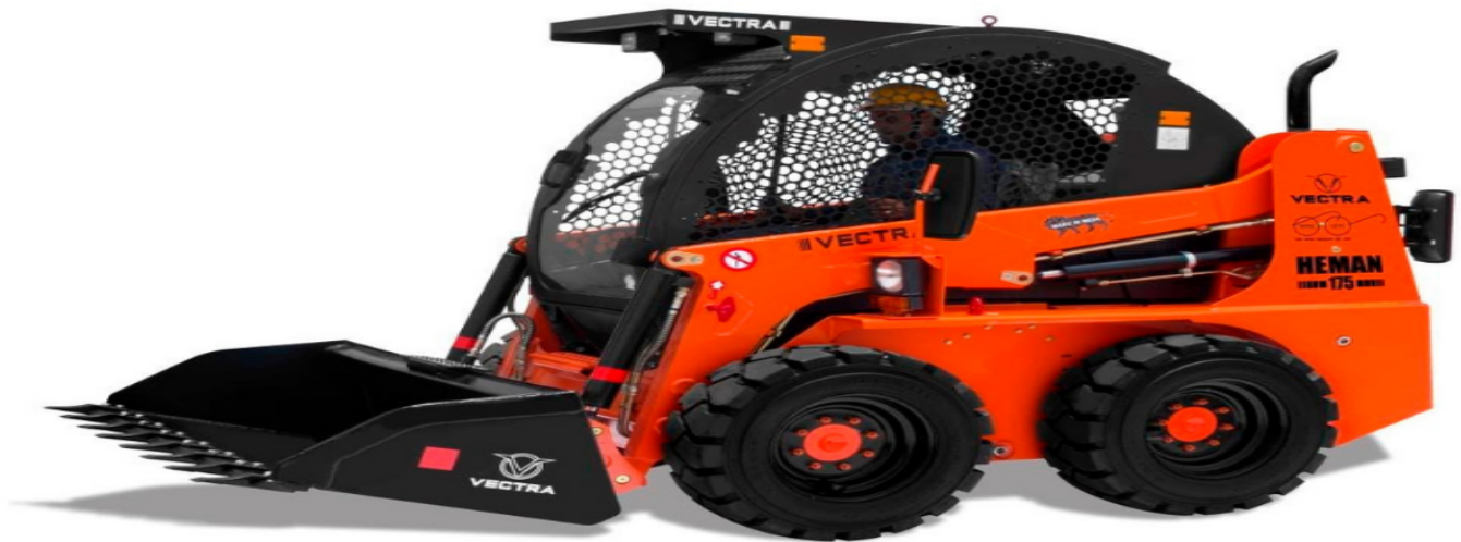
Heman 175 Skid Steer Loader ( With Standard Bucket ) Two Models Available BSIII-48HP / BSIV-72.5HP
