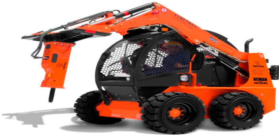
Heman 175 Skid Steer Loader ( With Rock Breaker ) Two Models Available BSIII-48HP / BSIV-72.5HP
